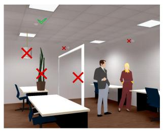
In order to improve the **Motion Detection**, it must be considered the higher sensitivity to tangential movements. Movements with radial direction are detected worse than tangential ones.
