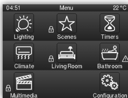
Figure 21. Menu with protection and alarms.
